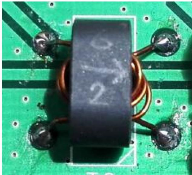
You will note that the schematic shows the multiple turn winding and the pads numbered one and two towards the IRF530 gates while the photos show a directional arrow to the right. The illustration above shows one turn to the right (IRF530 gates). I reasoned that the IRF530 gates are the low impedance side so I put the single turn winding to drive the gates.
